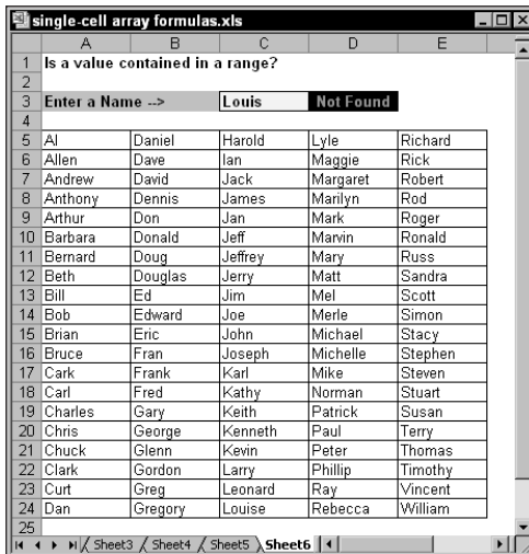
Figure 15-3: Using an array formula to determine if a range contains a particular value.
