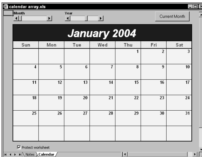
Figure 6-7: You can generate this calendar by using a single array formula, entered into 42 cells.
