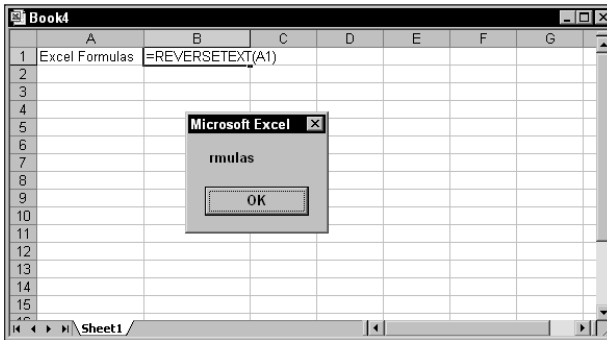
Figure 23-5: Use a MsgBox statement to monitor the value of a variable as a Function procedure executes.
